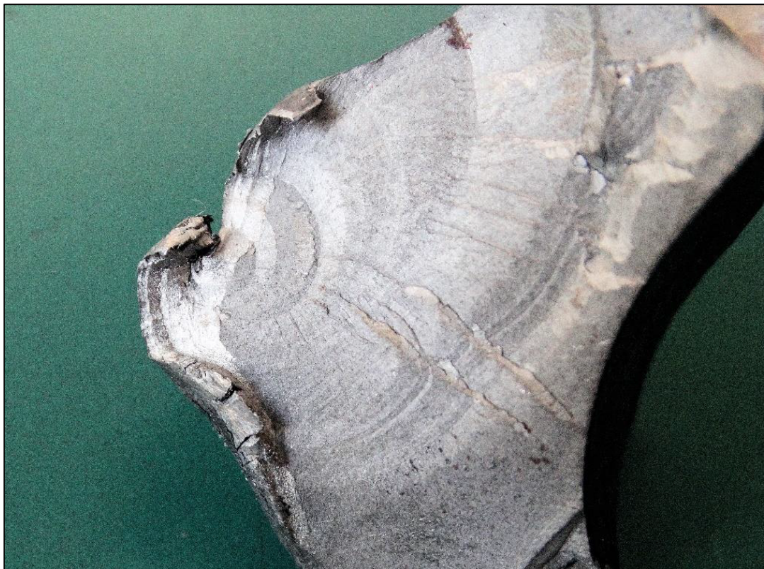
Photo 6. Initiation point after cleaning with Alconox®. Source: Force Technology.
