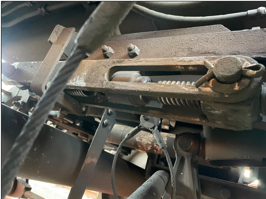
Photo 2. Hand brake actuator with threaded rod 8-9 revolutions from the end position.
