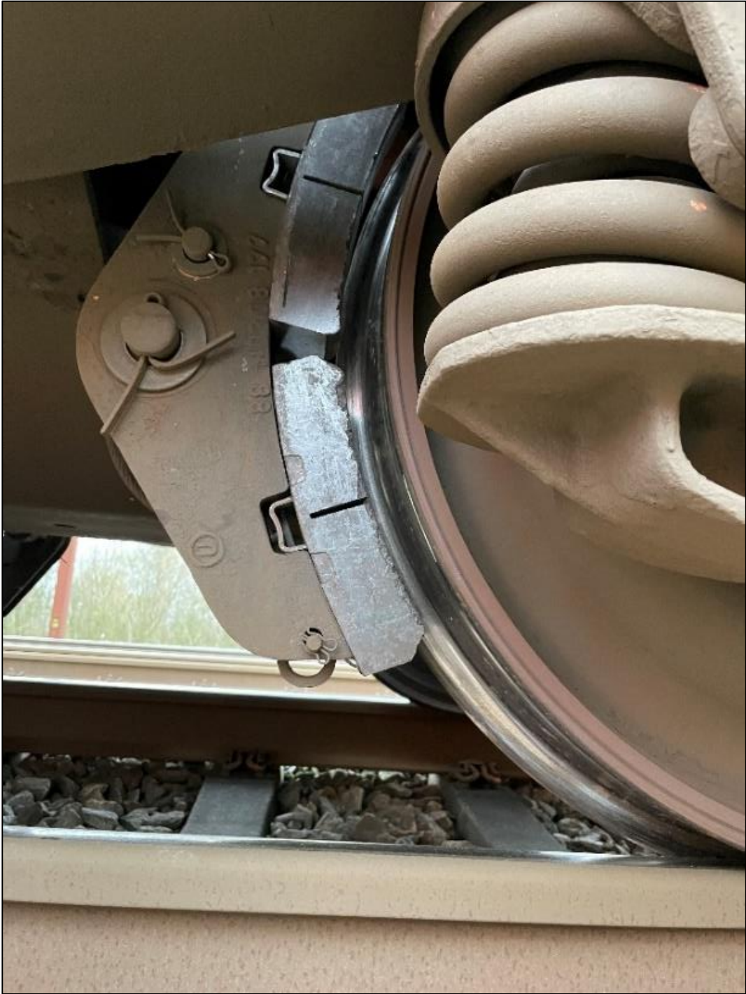
Photo 3. New brake blocks. The wagon's 3rd axle on the right-hand side.
