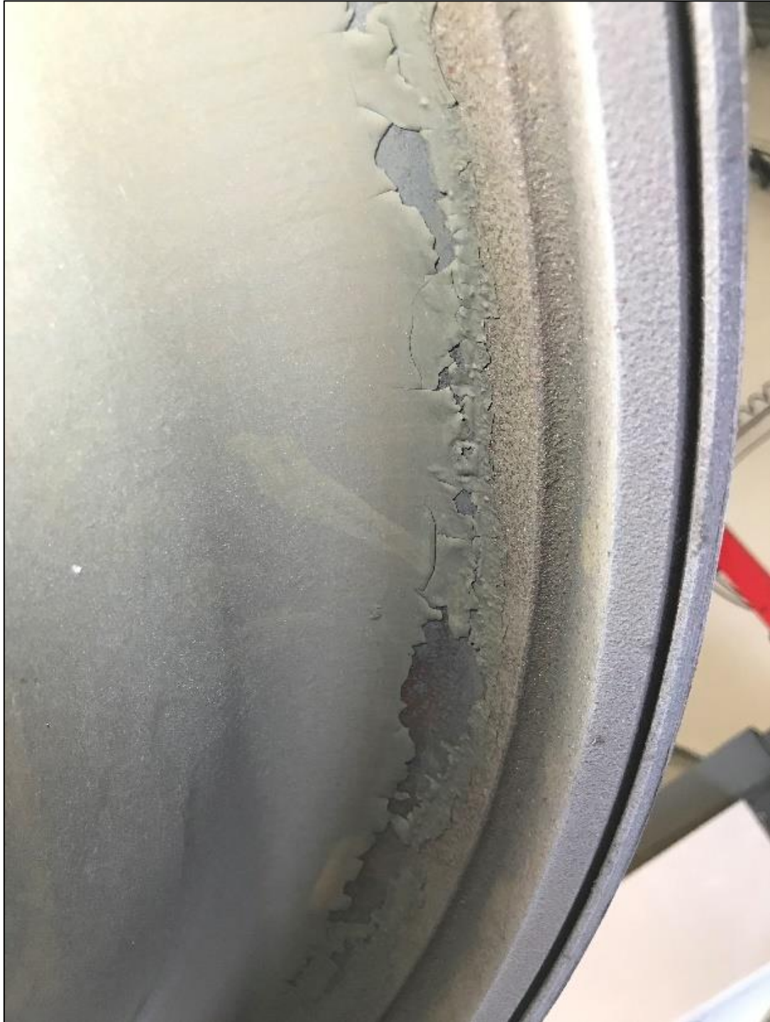
Photo 4. Burnt paint and corrosion in the transition between wheel plate and wheel rim.
