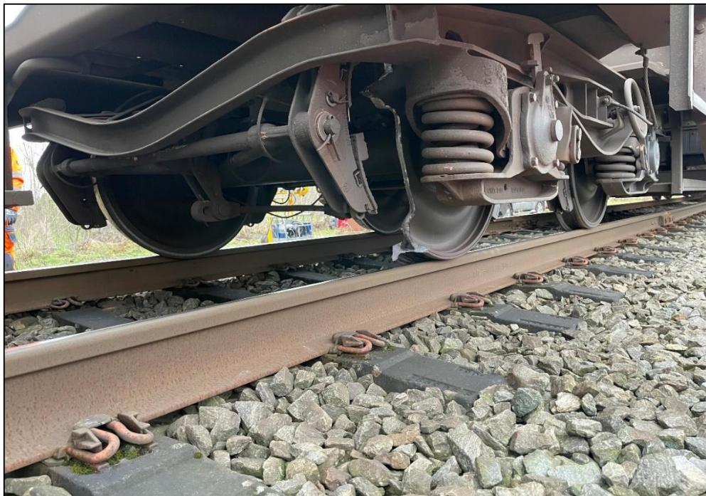
Photo 1. Axles 3 and 4 on the damaged wagon after stopping in Ejby.
