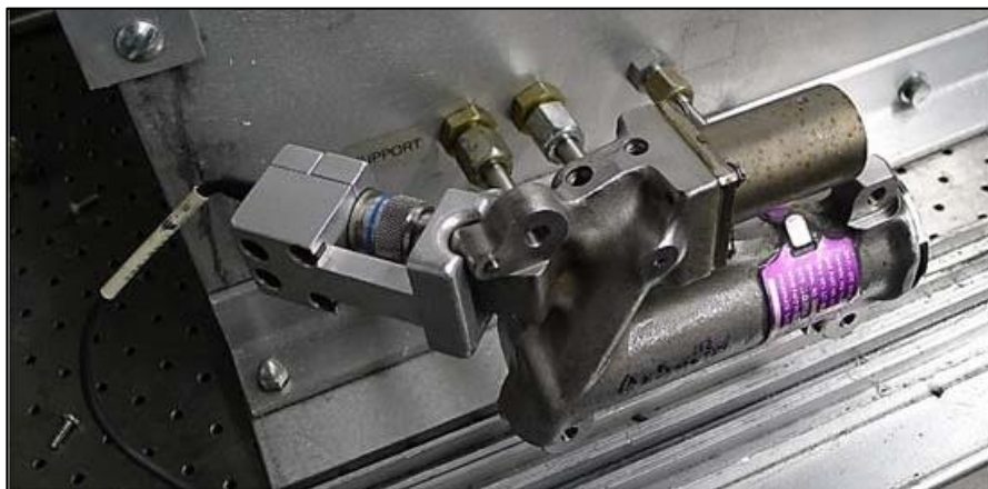
Figure 22. TRSOV in test rig
